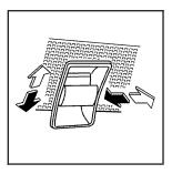
The sunroof control switch is located between the sun visors.
